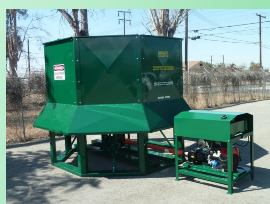
Fig. 9: Cold-Air-Drain Unit (SIS)
